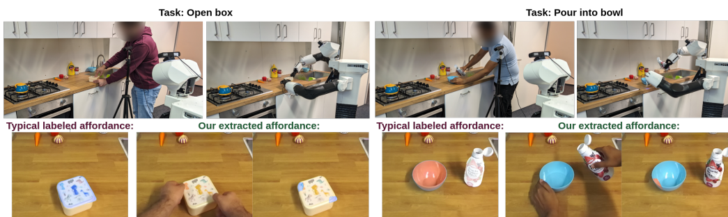
Figure 1: Examples of our affordance extraction in a real-world setting. The humans perform the tasks ‘open box’ and ‘pour into bowl’. With our affordance extraction method, we obtain the precise, actionable object regions used, which leads to downstream success when the robot executes the skill.
